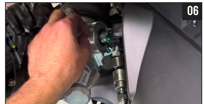
06 Remove sector shaft to the steering pinion pinch bolt (13mm). Mark the spline's alignment for reassembly.
