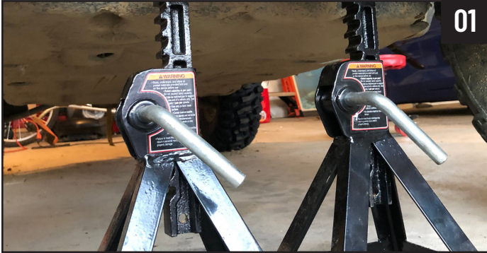
01 Safely raise and support the front end.
