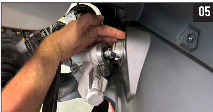
05 Cut the zip tie at the steering column boot and remove inner footwell plastic rivets to push the boot out of the way.
