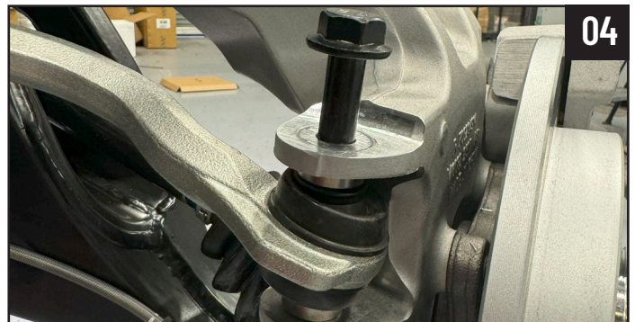
04 Remove both outer tie rod ends from the knuckles (18mm).
