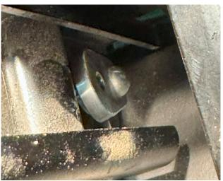
**6. IMPORTANT:** CAREFULLY Insert the new SANDCRAFT aluminum lower shift cable retainer over the cable and settle the shift cable end into the recessed ball cup. The flat side of the shift cable retainer faces forward. You can lay down a rag below the work area to catch it if it falls.
