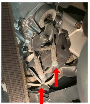
11. If there is play in the shift cable, you may need to tighten the shift cables at the transmission. Follow manufacturer specifications when adjusting shift cable tension (if needed). Re install the shift lever dust cover, gear selector cover and cupholders.
