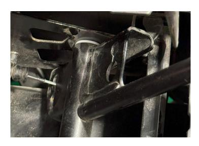
5. Push the lower shift cable through the large hole at the bottom of the shift bracket so it pushes through the shift bracket.
