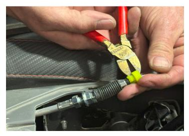
3. Cut the old plastic cable retainer away from the cable. Do not cut or damage the cable. This plastic component will not be reused.
