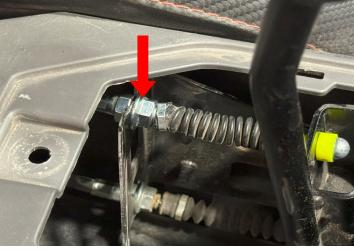
1. Chock the wheels to ensure the vehicle doesn't roll during installation. Remove the shift lever dust cover, gear selector cover and cupholders to expose the shift cable front assembly.
