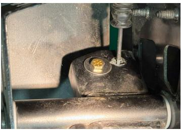
8. Once in place, apply blue threadlocker to the threads and insert the washer and screw to the back side of the shift bracket and torque to 20 in lbs.
