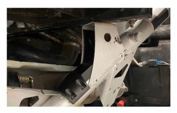
7. Raise and slide the passenger side bump stop up under the frame and trunk support pocket inserting the fork into the factory tie down knob.
