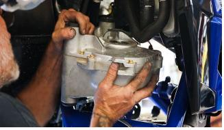
ONCE FRONT DIFF. IS INSTALLED, REINSTALL SUBFRAME INCLUDING PASSENGER & DRIVER SIDE PILLARS
