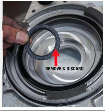
REMOVE ENGAGEMENT PLATE, ARMATURE PLATE, AND TORSION RING
