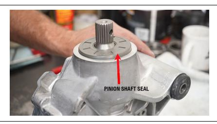
36 LET DIFF BE FILLED WITH 250 ML OF OIL ON BENCH AS TIME SAVER, BEFORE INSTALLING IT BACK INTO VEHICLE AND CAP VENT
