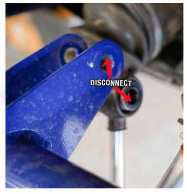
**REMOVE ELECTRICAL & VENT HOSE FROM DIFF BRACKET**
