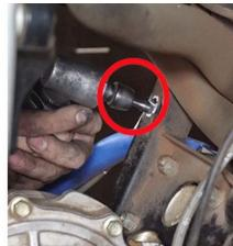
Slide in the RCR Stabilizer and line it up with the drilled holes onto frame. Then fit hardware into holes
