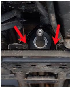
INSTALL THE 5/16TH BOLT THEN TORGUE ATTACH TO FRONT DIFF WITH SUPPLIED BOLT. TIGHTEN THE SUPPLIED FRONT DIFF REPLACEMENT BOLT. THEN TORQUE THE 2 ½" ALLEN SET SCREWS INTO THE FRONT DIFF INPUT SHAFT.
