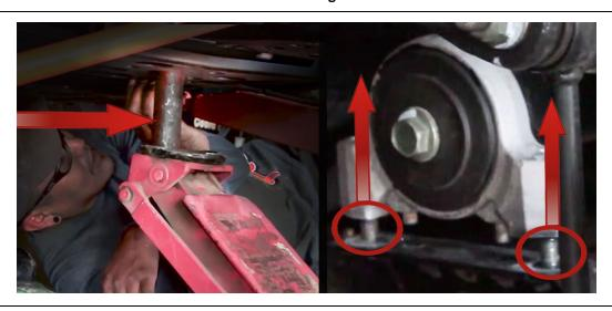
Remove the 2M 10 bolts (15mm socket) that are attached to the motor mount tube on each side, be sure to hold on to existing part as it will now be separated from machine.
