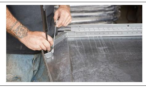
Install lower part of gas shock to trunk base
