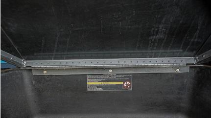
Tighten all hardware on hood but leave the bracket semi-loose
