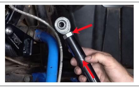
The slide plate is where the inner tie rod end retainer will go.
